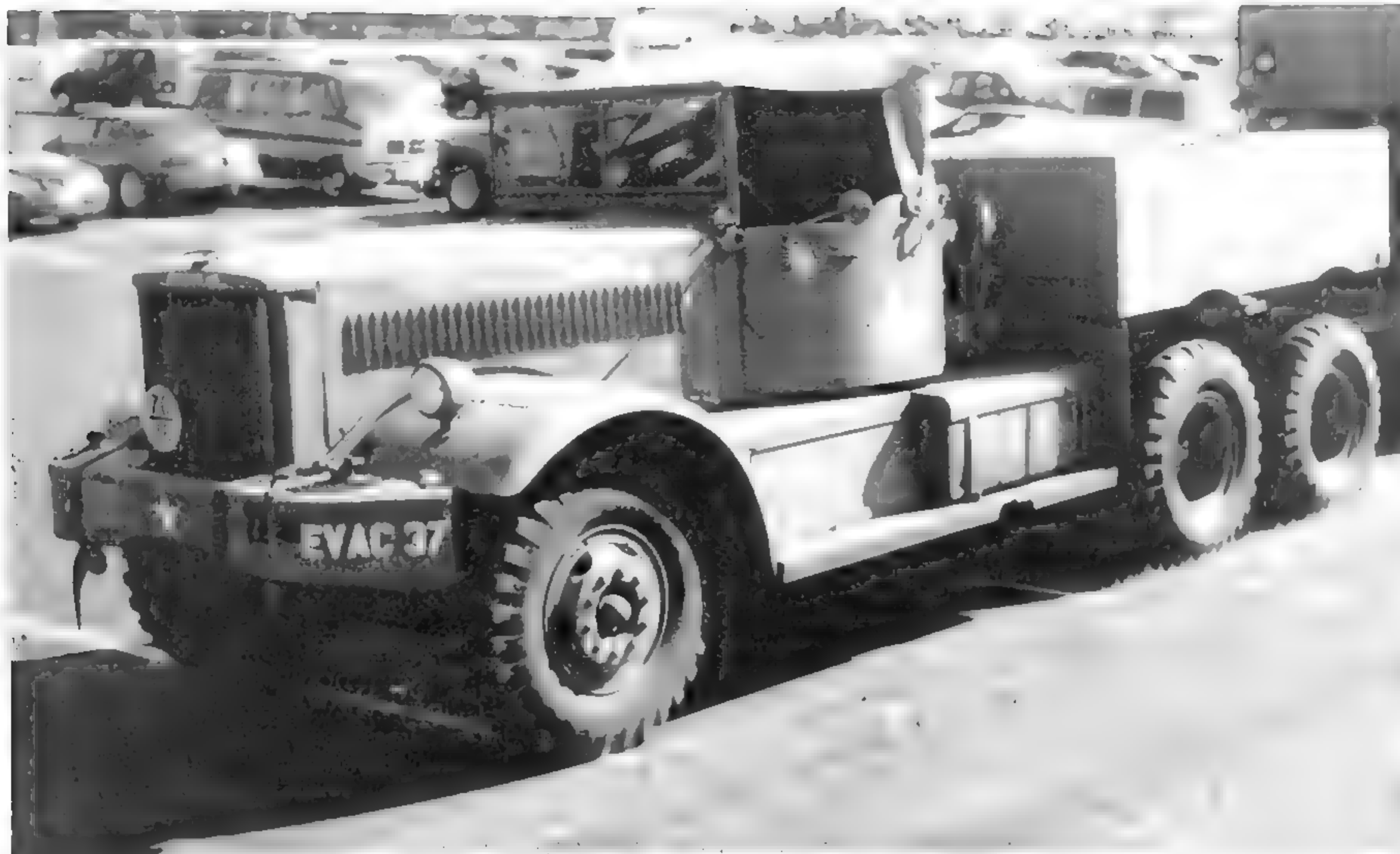
This restored 981 has the later-style open cab, and its ballast box has been filled with rock to increase traction.
